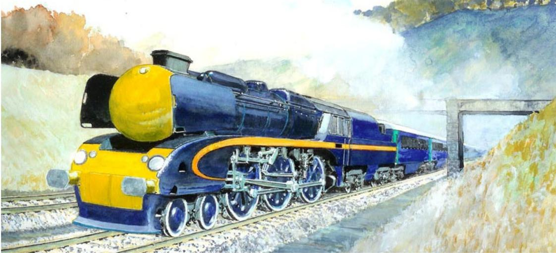
**The artist's final impression of the 5AT and how it would look running on the national network. Note the 'air dam' below buffer level. The front brake hoses and retractable coupling gear are pocketed when not in use. ROBIN BARNES**
