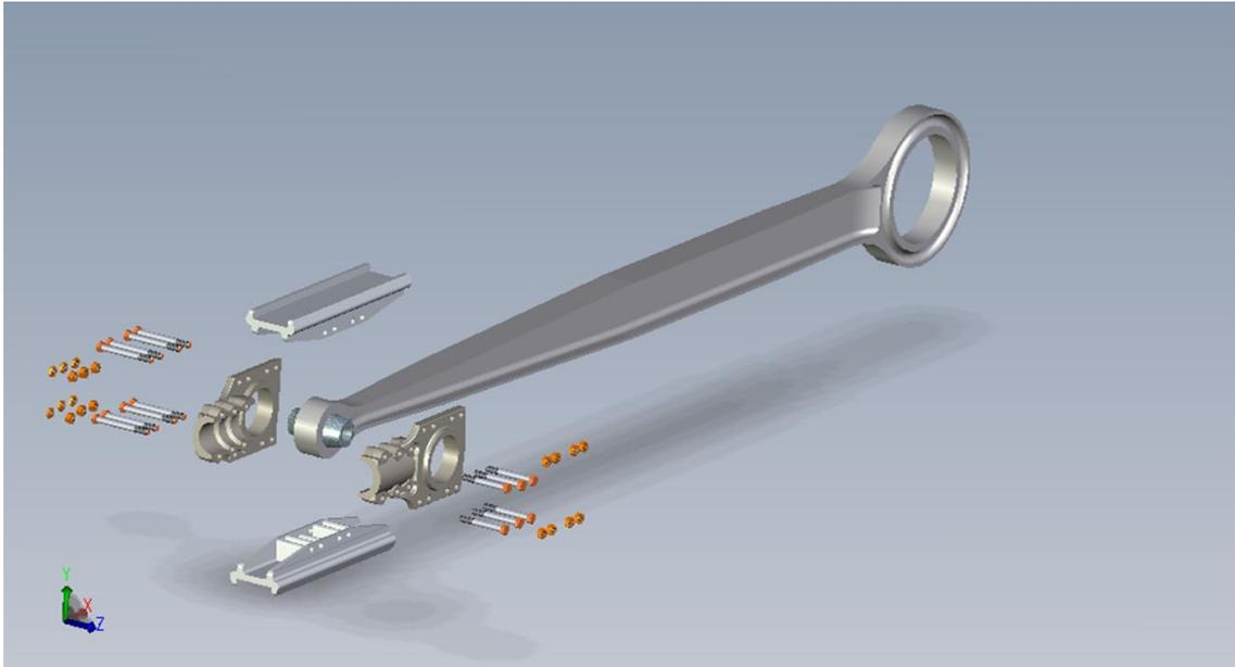
**Above: Computer Aided Design drawing of the 5AT's roller bearing connecting rod and some elements of the Timken-type split roller-bearing crosshead with aluminium alloy slippers. RICHARD COLEBY**
